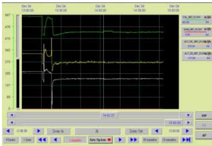
Figure 3.6 : Display of Flow x Time values during a leak trial. The position in time (14:02:27) of the leak is shown by the white line at the centre of the graph.
